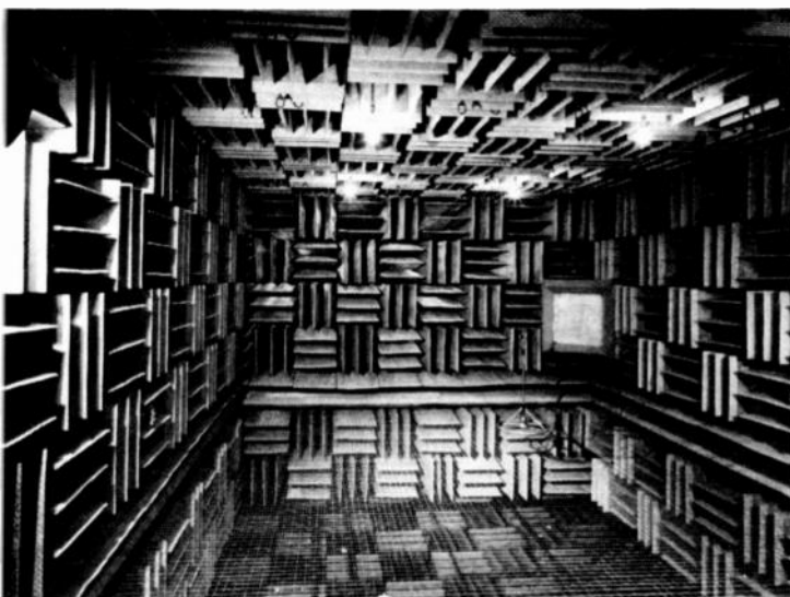
Though it is an important technical tool, not all speaker manufacturers have an anechoic chamber. This is E-V's.
