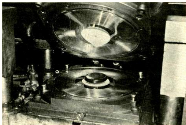
The press jaws, with record labels already in place, are about to close on a biscuit of extruded vinyl to mold a 12-inch disc.
