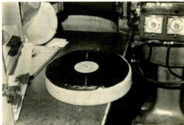
The final product, still warm from the press, awaits the operation that will trim the excess vinyl "flash" from its perimeter.
